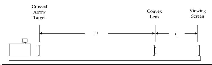
Complete the table on The Data Sheet. Using the data and the Fundamental Lens Equation determine a more accurate focal length of the Convex Lens. Also determine the magnification of the lens.
