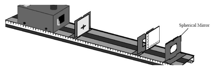
Complete the table on The Data Sheet. Using the data and the Fundamental Lens Equation determine a more accurate focal length of the spherical mirror. Also determine the magnification of the mirror.
